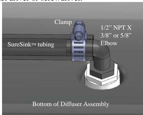
7. Install strain relief over tubing and secure to diffuser base as shown using 7/16" socket and wrench. A properly installed strain relief will prevent any damage to the diffuser assembly when it is lowered in the water or pulled up at a later date for maintenance.
