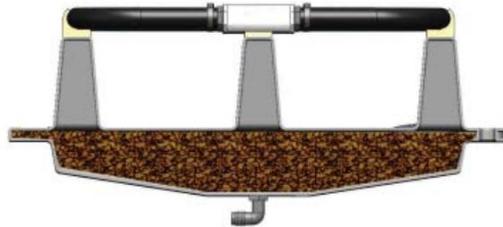
3. Install vent plug once base is completely full.
