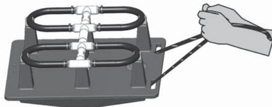
13. While holding the two ends of the rope, gently lower the diffuser assembly into the water. Submerge the assembly and allow the air to escape from the vent plug as the base fills with water.
